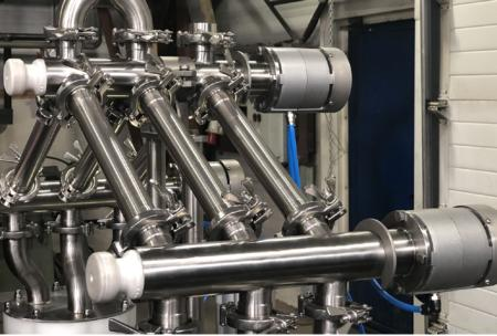
The ice cream dispenser consists of a rack, bracket, flow distributors, connecting pipes, tee.
